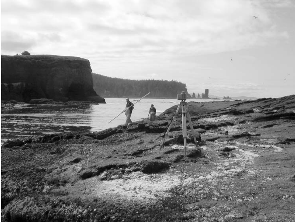
PLATE 1. Measurements of intertidal heights were conducted at most sites with a laser level, using a reference point obtained by observing still tidal height on multiple days. The site shown here is Strawberry Draw, Tatoosh Island, Washington, USA. Photo credit: B. Helmuth.
